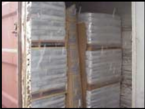
Bagged product unitized with stretch wrap, loaded on pallets three high with a DID bag in the center void.
